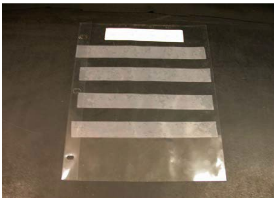
Figure 10 - Tape lift collections placed onto a sheet protector.
